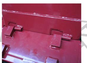
10.Install discharge chute following the same procedure as the Feed hopper ensuring the two retaining bolts are fitted and fully tightened once it is in position.
